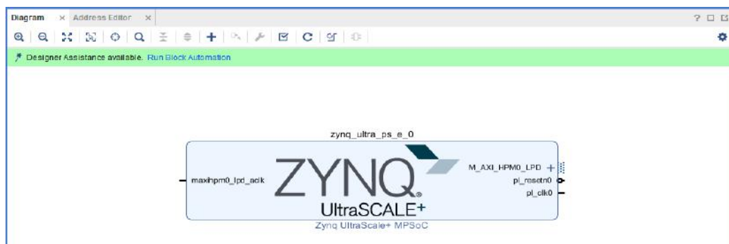
Figure 2-2: Zynq UltraScale+ MPSoC Processing System IP Block
