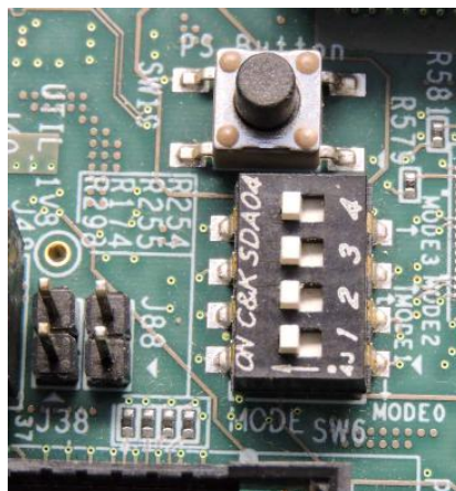
Figure 4-4: SW6 Switch Settings for JTAG Boot Mode
