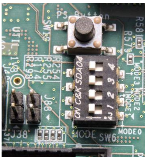
Figure 5-26: SW6 Switch Settings for JTAG Boot Mode
