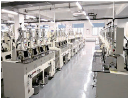
Fully-auto Polishing machine
