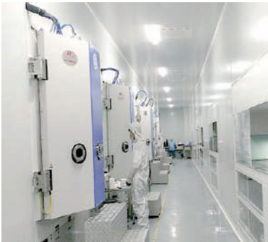
Optical thin film coater
