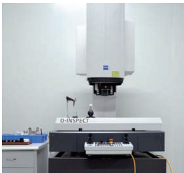
Coordinate measuring machine
