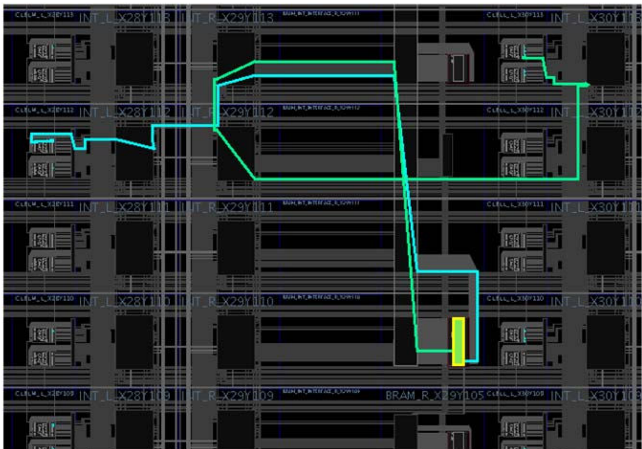
Figure 5-21: Example: Routing to and from a Block RAM
