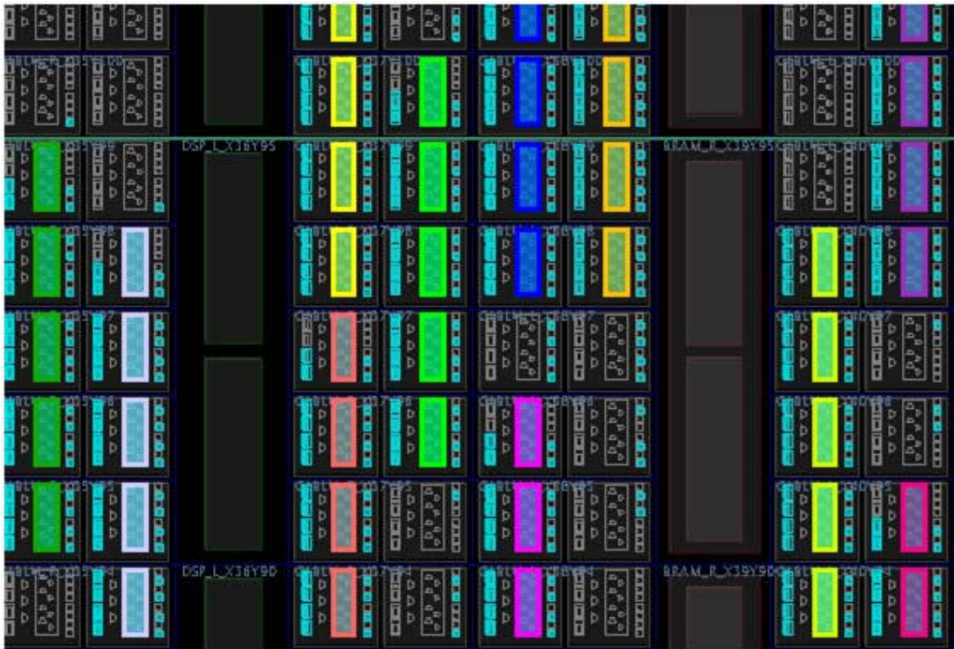
Figure 5-25: DSP48 Implemented in CLBs
