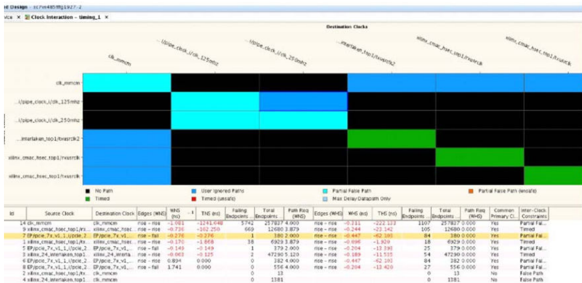
Figure 5-7: Sample Clock Interaction Report
