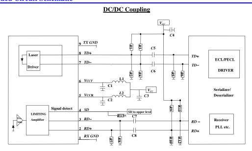
C1/C2/C4/C5/C6/C7/C8 = 100 nF $R1/R3 = 82\Omega$   $C3 = 4.7 \ \mu\text{F}$  $R2/R4 = 130 \ \Omega$
