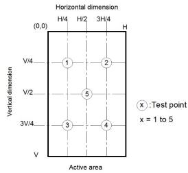
Light spot size ∅=7mm, 500mm distance from the LCD surface to detector lens measurement instrument is TOPCON's luminance meter BM-7
