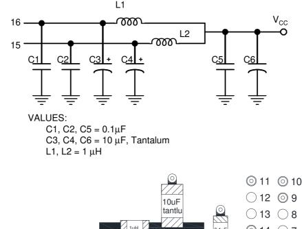
12 <a>\text{ } 9 ○ 13 ○ 8 1uH ( ) 15 ( ) 6 ○ 16 ○ 5 0.1uF 10uF tantlu  $\bigcirc$  18  $\bigcirc$  3 10uF tantlu  $\bigcirc$  19  $\bigcirc$  2 Connected to Vcc O Connected to GND © 20 © 1  $\odot$
