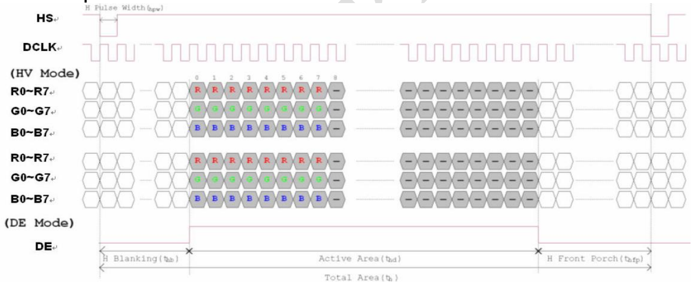
Fig. Horizontal input timing diagram
