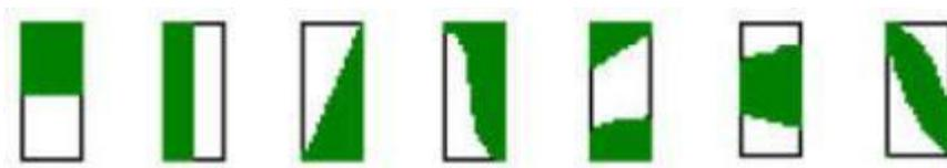
3.8 A dot defect that is smaller than the defined dot defect will be treated as small bright dot. 细碎亮点：小于“DOT 定义”的点缺陷视为细碎亮点。
