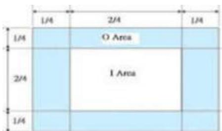
3.9 Inspection method of ND Filter - holding ND filter in front of the panel around 5cm and examine the panel from 35±5 cm in the front view for 2~3 second.
