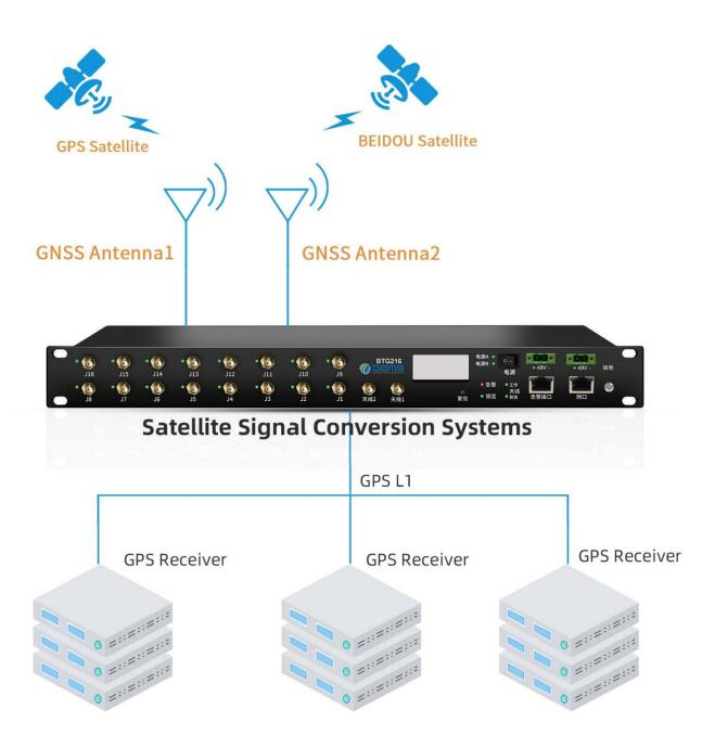
Timing devices that do not support BeiDou satellite signals, such as some of the early construction of BBU or other timing systems.
