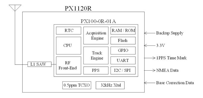
Active antenna is required to use with PX1120R. The received signal goes through a L1 SAW filters to remove out-band interference, then to the PX100 GNSS receiver chip for RTK signal processing. Using correction data from an RTK base station, the rover PX1120R computes its position to centimeter-level accuracy relative to the base station.
