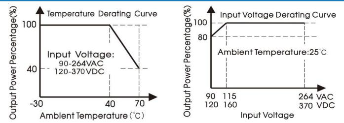
Note: ①With an input voltage between 90 -115VAC and a DC input between 120-160VDC the output power must be derated as per the temperature derating curves;
