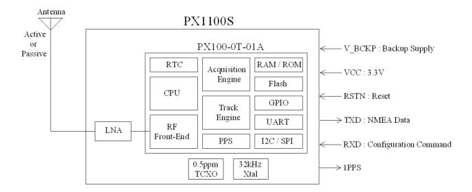
The PX1100S is a L1 quad constellation capable satellite navigation receiver in a compact surface mount package. It is based on the latest single-chip Phoenix GNSS receiver technology, providing high performance signal acquisition and tracking. The simple UART serial interface and the standard NMEA-0183 protocol make usage of PX1100S very easy and straightforward.
