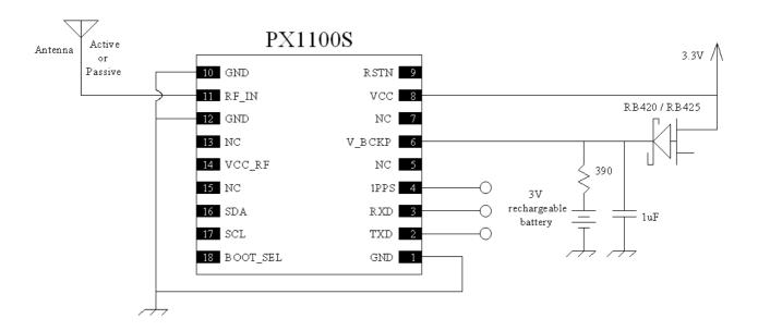
When PX1100S has previously been used within 2 hour, for faster time to first fix powering up without needing to decoded ephemeris data from signal, V\_BCKP should be connected to non-volatile supply; above figure with V\_BCKP connected to rechargeable battery is an example implementation. If cold starting every time powering up is not an issue, V\_BCKP can be connect to VCC.
