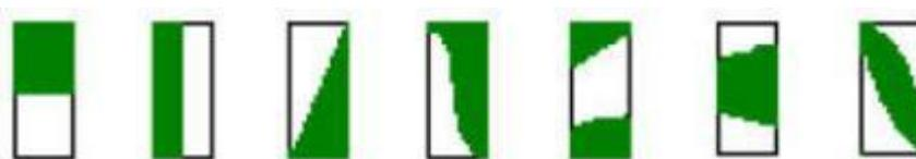
3.8 A dot defect that is smaller than the defined dot defect will be treated as small bright dot. 细碎亮
