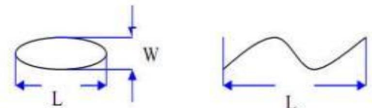
3.5 When defect size  $L \geq 2W$ , the defect count as liner type defect. Size of linear defect is defined by length(L) and the maximum width(W).
