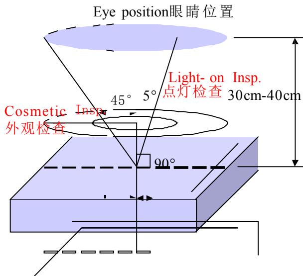
(Perpendicular to LCD panel surface 垂直于液晶显示表面)
