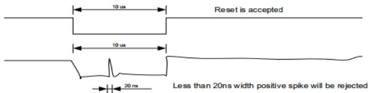
Figure 125: Positive Noise Pulse during Reset Low
