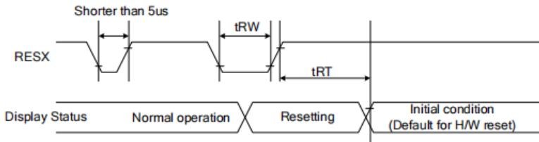
Figure 124: Reset Timing
