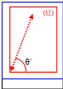
CF side polarizing absorption angle  $\theta=15^\circ$  (Protective film on top, glue layer face down)
