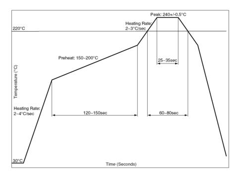
The reflow profile shown above should not be exceeded, since excessive temperatures or transport times during reflow can damage the module. Cooling temperature fall rate: max 3°C / sec
