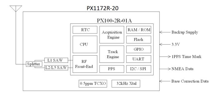
Active antenna is required to use with PX1172R-20. The received signal goes through a signal splitter, to individual L1 and L2/L5 SAW filters to remove out-band interference, then to the PX100 GNSS receiver chip for RTK signal processing. Using correction data from an RTK base station, the rover PX1172R-20 computes its position to centimeter-level accuracy relative to the base station.
