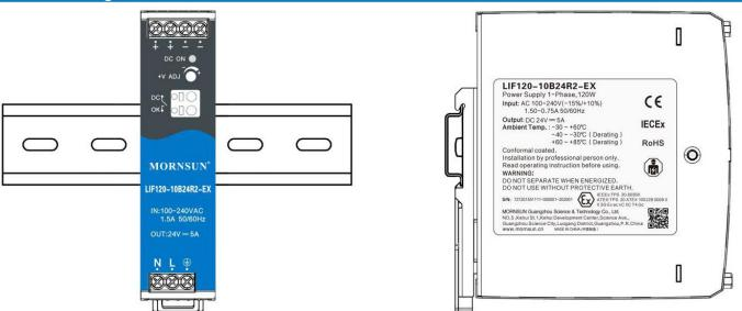
Notice: Keep the following installation clearances: 20mm on top, 20mm on the bottom, 5mm on the left and right sides are recommended when the device is loaded permanently with more than 50% of the rated power. Increase this clearance to 15mm in case the adjacent device is a heat source (e.g. another power supply).
