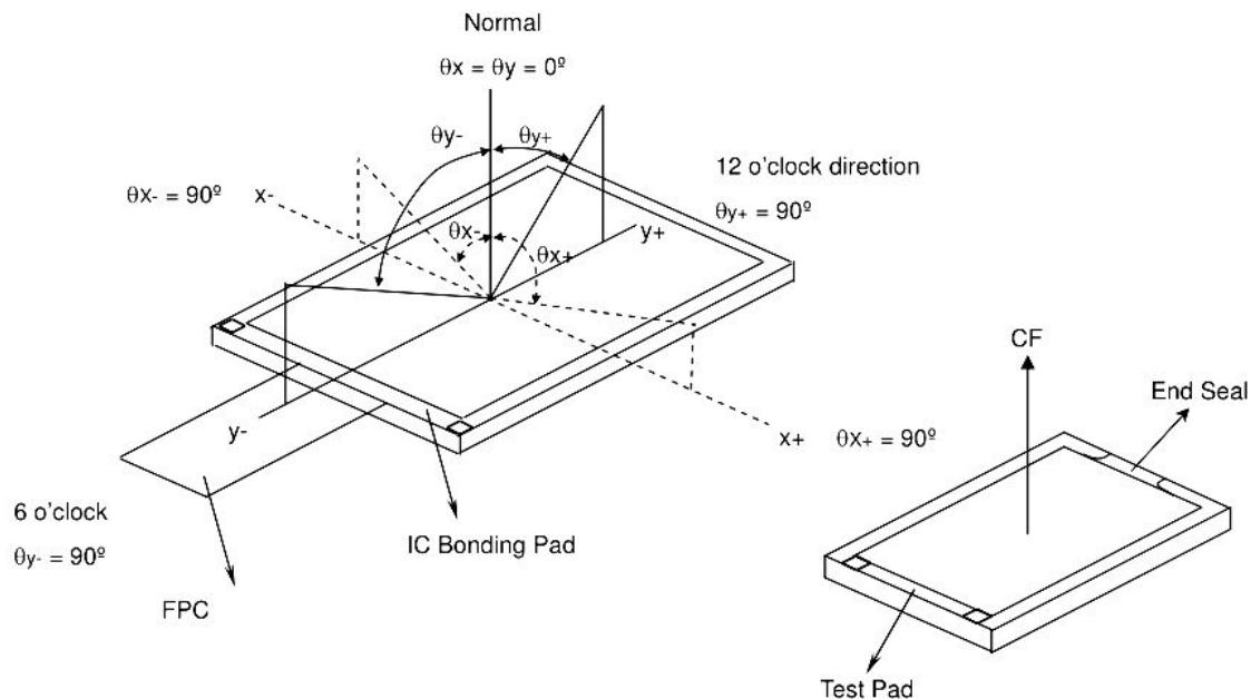
Note 6. The LCD module should be stabilized at a given temperature for 20 minutes to avoid abrupt temperature change during measuring. In order to stabilize the luminance, the measurement should be executed after lighting Backlight for 20 minutes in a windless room. Measuring method for Contrast ratio, surface luminance, Luminance uniformity,CIE(x,y) chromaticity.
