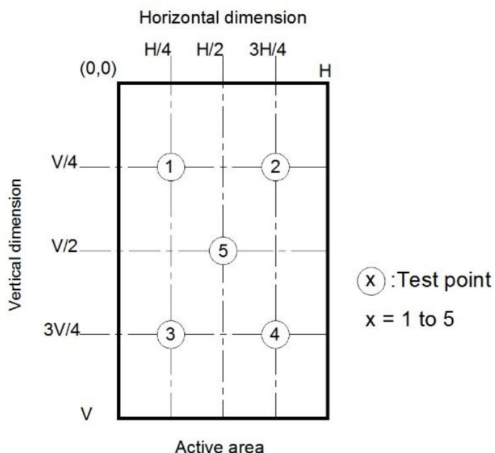
Light spot size  $\phi = 7\text{mm}$ , 500mm distance from the LCD surface to detector lens
