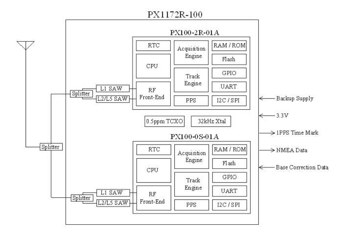
Active antenna is required to use with PX1172R-100. The received signal goes through a signal splitter, to individual L1 and L2/L5 SAW filters to remove out-band interference, then to the PX100 GNSS receiver chip for RTK signal processing. Using correction data from an RTK base station, the rover PX1172R-100 computes its position to centimeter-level accuracy relative to the base station.
