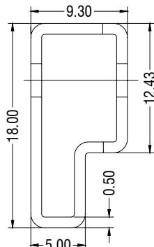
Tube length (14 Pin DIP) : 520mm $\pm$ 2mm.
