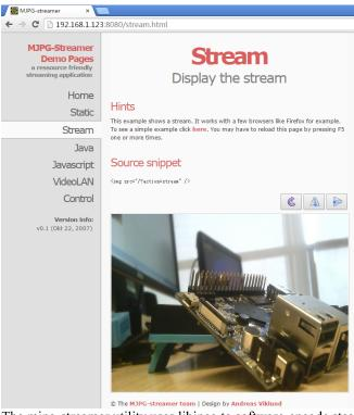
The mjpg-streamer utility uses libjpeg to software-encode steam data. The Linux-4.14 based ROM currently doesn't support hardware-encoding. If you use a H3 boards with Linux-3.4 based ROM you can use the ffmpeg utility to hardware-encode stream data and this can greatly release CPU's resources and speed up encoding:
