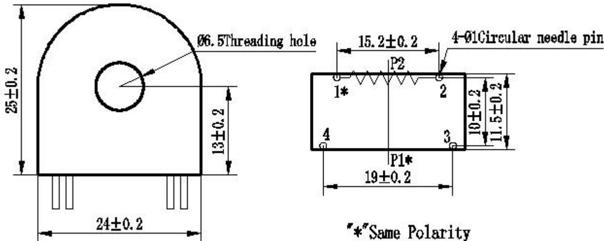
Remarks: Primary input: straight- through type( make the measured circuit be through the hole)
