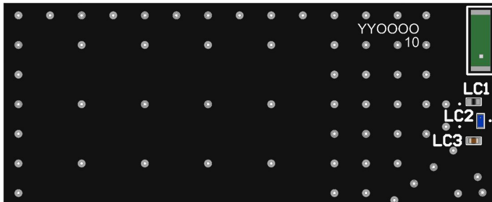
3D View of matching components and recommended values (LC1 = OPEN, LC2=3.6nH, LC3= 1.2pF)
