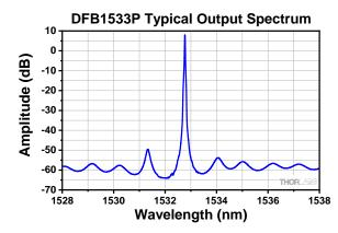
The spectrum was measured using an optical spectrum analyzer with a spectral resolution of 0.02 nm.
