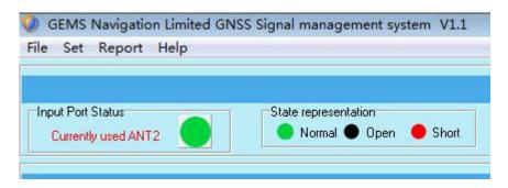
If the antenna open or short circuit, the front panel of the machine GPS Locked green light is off, Alarm red light flashes to indicate alarm, PC-side reading antenna operating state shorted or opened.
