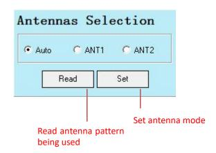
Active antenna mode select: Select "AUTO" or other antenna patterns Click "Set" prompt setup is successful, while the unit's front panel LCD displays the antenna pattern used in this case, if you select "AUTO" mode the unit's front panel "ANT1" bright blue light, select "ANT1" mode is "ANT1" lights up in blue, select "ANT2" mode "ANT2" lights up in blue, the active antenna selection mode can also be operated in the front panel
