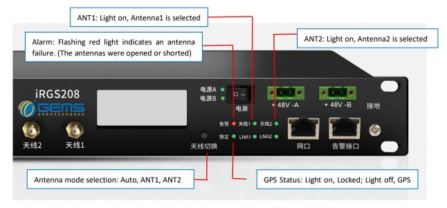
"AUTO" mode: automatic selection mode for the antenna when switching to this mode will automatically turn access antennas 1 and 2 compare the signal strength and then select a better signal antenna access. In this mode the device automatically switches the antenna will be delayed.
