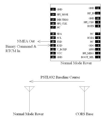
For Precise Heading, Moving Base Mode Configuration
