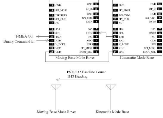
For Precise Positioning & Heading, Advanced Moving Base Mode Configuration #1
