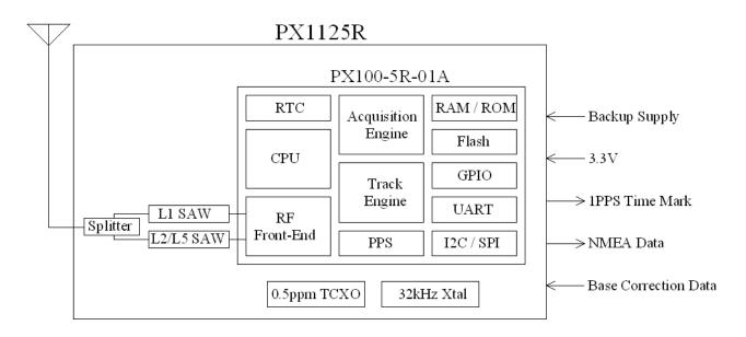
Active antenna is required to use with PX1125R. The received signal goes through a signal splitter, to individual L1 and L2/L5 SAW filters to remove out-band interference, then to the PX100 GNSS receiver chip for RTK signal processing. Using correction data from an RTK base station, the rover PX1125R computes its position to centimeter-level accuracy relative to the base station.
