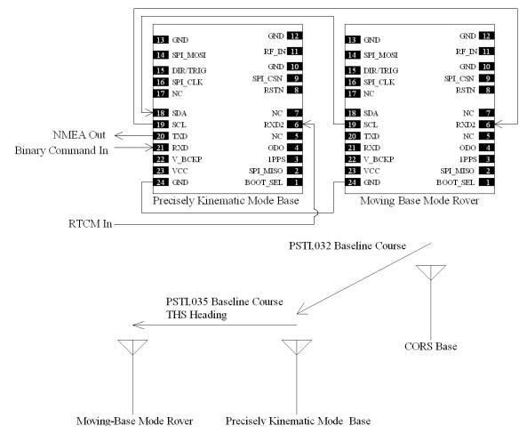
For Precise Positioning & Heading, Advanced Moving Base Mode Configuration #2
