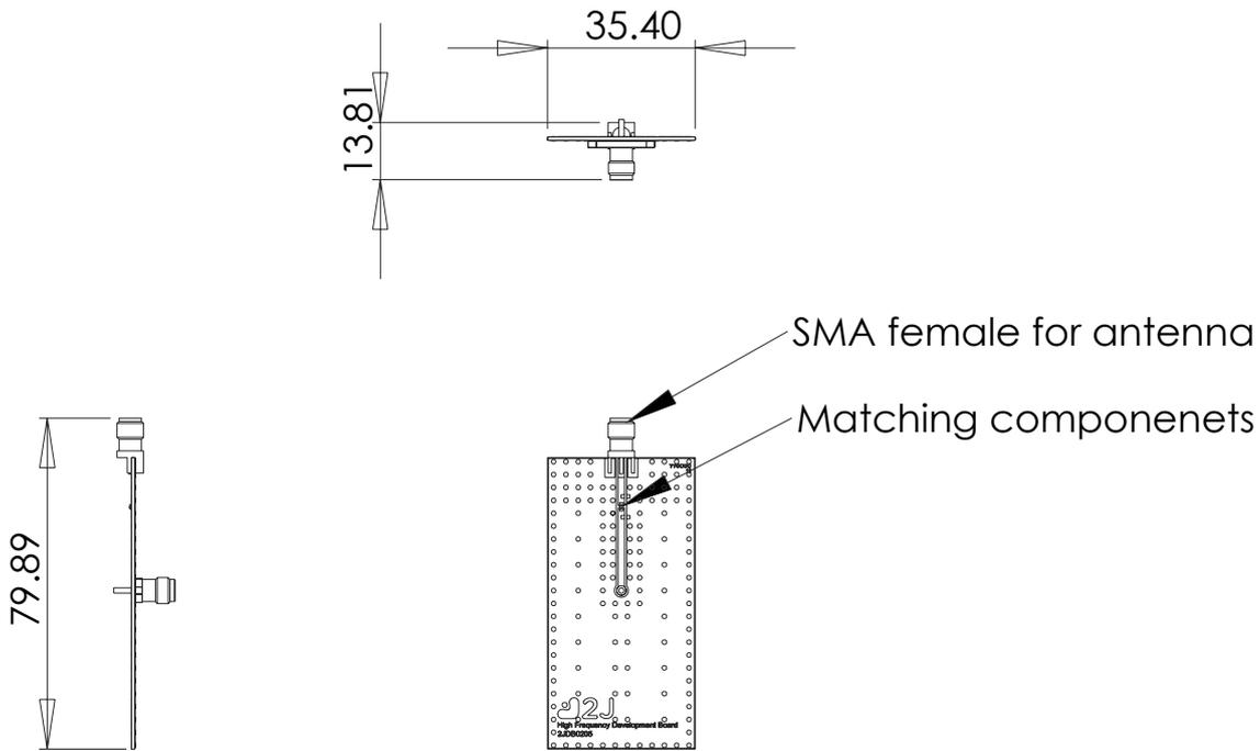
This development board is suitable for finding best matching componenets for high frequency antennas and test high frequency antenna as ground size is similar to most of the existing devices on market.
