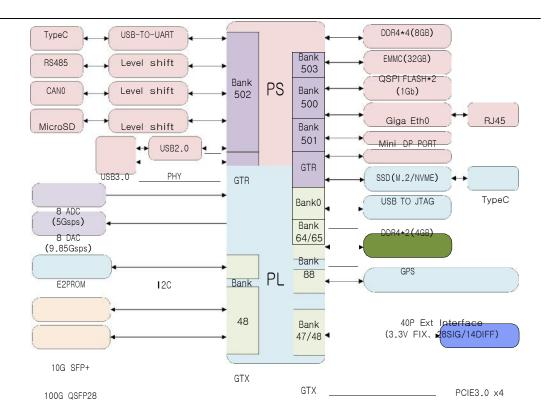
The interfaces and functions included in the RF SOC development platform are as follows:
