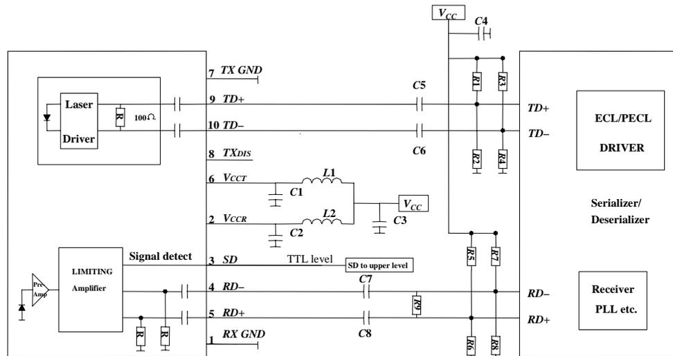
$C1/C2/C4/C5/C6/C7/C8 = 100 \text{ nF}$        $C3 = 4.7 \mu\text{F}$        $L1/L2 = 1 \mu\text{H}$
