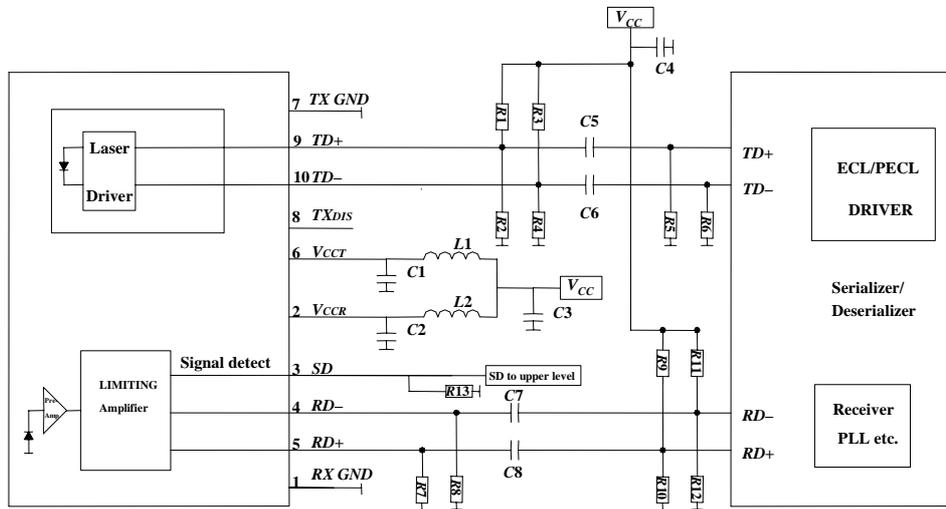
$C1/C2/C4/C5/C6/C7/C8 = 100 \text{ nF}$        $C3 = 4.7 \mu\text{F}$        $L1/L2 = 1 \mu\text{H}$
