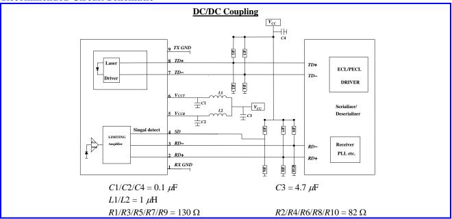
In order to get proper functionality, a recommended circuit is provided in above recommended circuit schematic. When designing the circuit interface, there are a few fundamental guidelines to follow.
