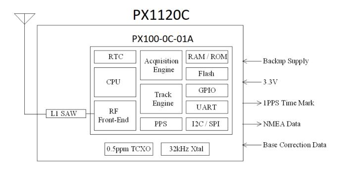
Active antenna is required to use with PX1120C. The received signal goes through a L1 SAW filters to remove out-band interference, then to the PX100 GNSS receiver chip for signal processing.
