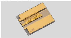
SkyEra delivers TY -808 $\pm$ 3nm-5.0W-25C-COS-200 chip on submount diode lasers, employing AuSn bonding and P Down package with multiple advantages of high reliability, stable output power, high power, high efficiency, long lifetime and high compatibility, and are widely applied in the market.
