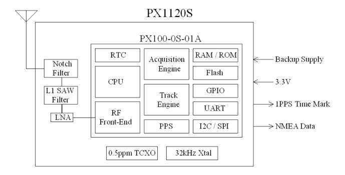
The PX1120S is a high performance L1 quad constellation capable satellite navigation receiver in a compact surface mount package. It is based on the latest single-chip Phoenix GNSS receiver technology, providing high performance signal acquisition and tracking. The simple UART serial interface and the standard NMEA-0183 protocol make usage of PX1120S very easy and straightforward.
