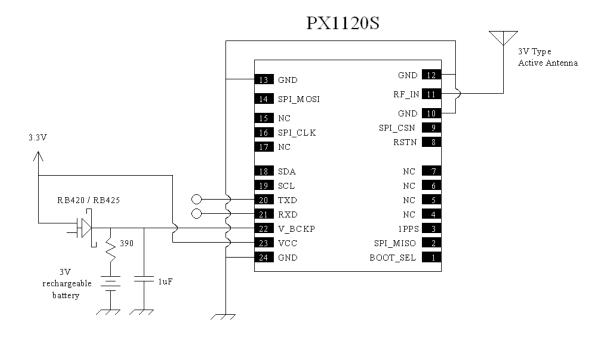
When PX1120S has previously been used within 2 hour, for faster time to first fix powering up without needing to decoded ephemeris data from signal, V\_BCKP should be connected to non-volatile supply; above figure with V\_BCKP connected to rechargeable battery is an example implementation. If cold starting every time powering up is not an issue, V BCKP can be connect to VCC.
