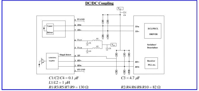
In order to get proper functionality, a recommended circuit is provided in above recommended circuit schematic. When designing the circuit interface, there are a few fundamental guidelines to follow.
