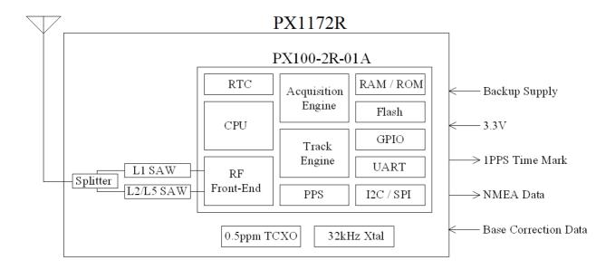
Active antenna is required to use with PX1172R. The received signal goes through a signal splitter, to individual L1 and L2/L5 SAW filters to remove out-band interference, then to the PX100 GNSS receiver chip for RTK signal processing. Using correction data from an RTK base station, the rover PX1172R computes its position to centimeter-level accuracy relative to the base station.
