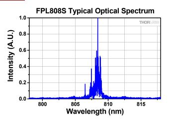
While the laser diode was held at 25 °C, it was driven at the current required to reach an output power of 250 mW.
