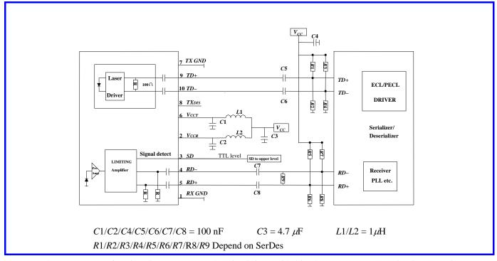
In order to get proper functionality, a recommended circuit is provided in above recommended circuit schematic. When designing the circuit interface, there are a few fundamental guidelines to follow.
