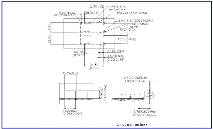
This transceiver is compatible with industry standard wave or hand solder processes. After wash process, all moisture must be completely remove from the module. The transceiver is supplied with a process plug to prevent contamination during wave solder and aqueous rinse as well as during handling, shipping or storage.
