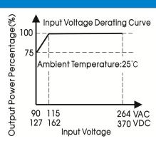
Note: 1.With an AC input voltage between 90-115VAC and a DC input between 127-162VDC the output power must be derated as per the temperature derating curves:
